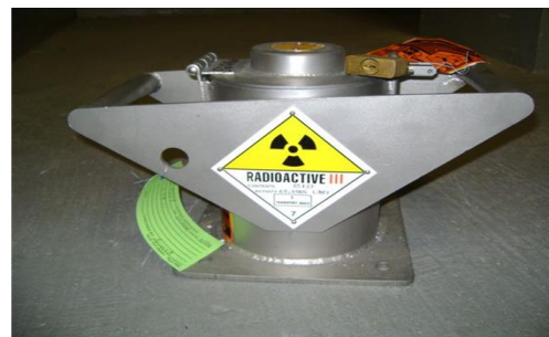
Figure 2. Representative shielded containers, neutron on left and density on right (Figures courtesy of Halliburton and adopted from Badruzzaman et al., 2009).
