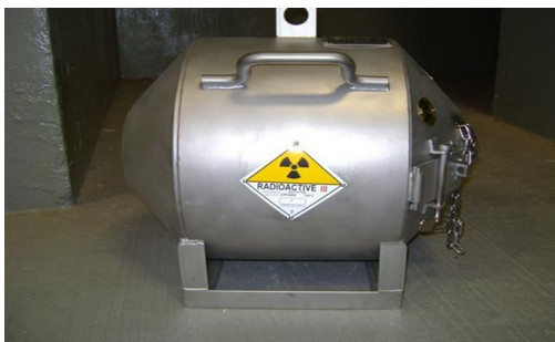
Figure 2. Representative shielded containers, neutron on left and density on right (Figures courtesy of Halliburton and adopted from Badruzzaman et al., 2009).
