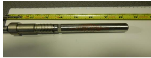
Figure 1b. An ^{241}\text{Am-Be} neutron porosity source capsule (Hearn, 2014)
